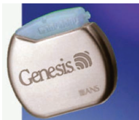
Figure 221-1 Internal pulse generator. (Courtesy of Advanced Neuromodulation Systems, Inc./St. Jude Medical, St. Paul, MN.)
