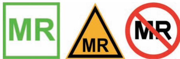
Figure 170-2 Signs and labels used to designate magnetic resonance (MR) zones. Green: safe in zone IV, nonmagnetic, nonelectrically conductive, and non-radio-frequency reactive. Yellow: may contain magnetic, electrically conductive, or radio-frequency-reactive components and is usually labeled for safe operation within fields below a certain strength (e.g., <500 gauss or <5 gauss). Red: unsafe because it contains ferromagnetic material and, therefore, has the potential to harm patients or equipment if brought into zone III or IV.
