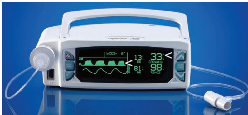
Figure 8-1 ● Waveform capnographer, displaying the \text{ET CO}_2 value (<) with each breath and a waveform (<) representing exhaled \text{CO}_2 concentration over time.
