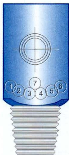
Fig. 2.8: Cylinder valves showing position of holes (these holes correspond to same pins at yoke of machine)
