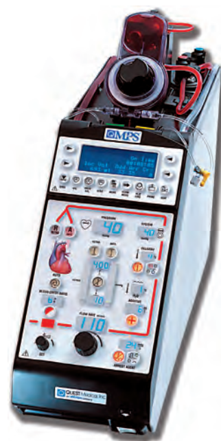
Fig. 32.31 Quest Myocardial Protection System (MPS). Cardioplegia is pumped by a system actuated by a stepper motor. Arrest solution and additive solutions are contained in 50-mL pouches and may be precisely added to the delivery solution. The disposable heat exchanger component is attached to the top of the console. The MPS has system and delivery pressure sensors, as well as an air detection and elimination system. Blood-to-crystalloid ratio, temperature, and additive drug concentrations may be adjusted in real time during delivery. (Courtesy Quest Medical, Allen, TX.)
