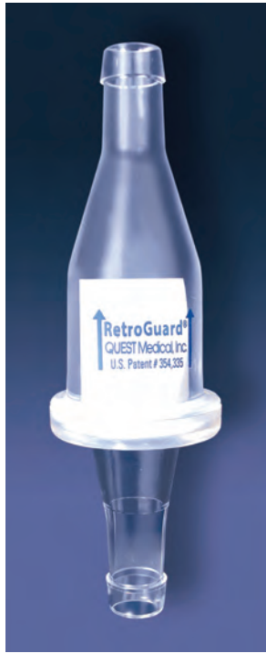
Fig. 32.9 Quest Medical RetroGuard Valve. Blood enters from the 3/8-inch inlet, passes through a duck-billed valve, and exits through a 3/8-inch outlet. This valve prevents retrograde flow. This valve may also be placed on an inlet port of the venous reservoir to prevent pressurization of the hard shell venous reservoir. (Courtesy Quest Medical, Allen, TX.)
