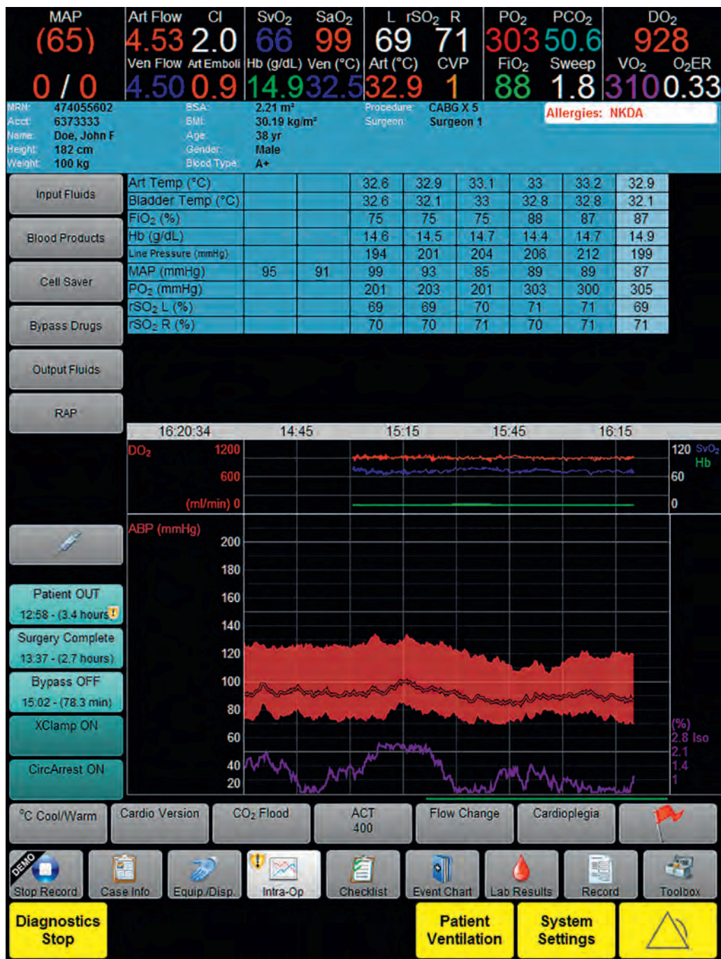
Fig. 32.10 Viper display with table and graphical display of data. (Courtesy of Spectrum Medical, Fort Mill, SC.)
