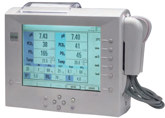
Fig. 32.39 CDI500 continuous blood gas and saturation monitor. Measures arterial and venous pH, \text{PCO}_2 , \text{PO}_2 , potassium, hemoglobin saturation, hematocrit, and hemoglobin. (Courtesy Terumo Cardiovascular Group, Ann Arbor, MI.)
