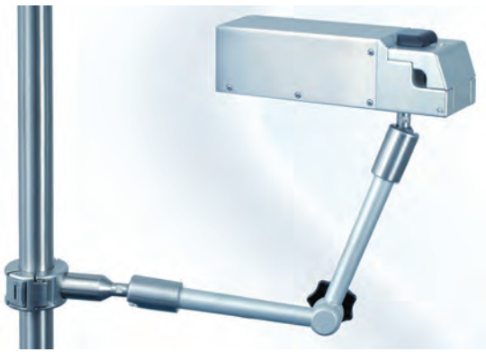
Fig. 32.8 E-Clamp electronic line clamp works in conjunction with the Revolution centrifugal pump. The clamp is automatically deployed to clamp the line when retrograde flow is detected or if the air detector or level detector is triggered. (Courtesy Sorin Group, Arvada, CO.)
