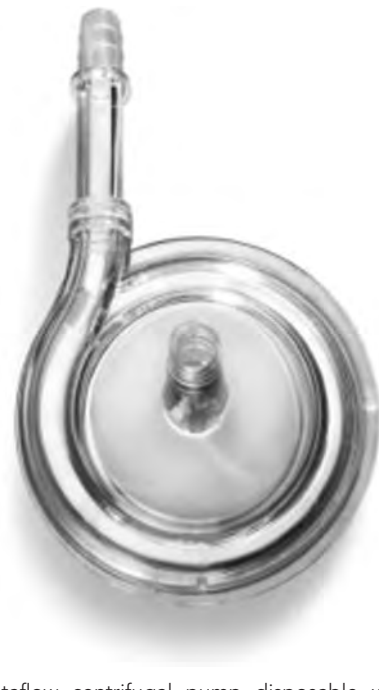
Fig. 32.4 Rotaflow centrifugal pump disposable with low-friction one-point bearing (sapphire ball and PE calotte). (Courtesy Maquet Cardiovascular, Wayne, NJ.)
