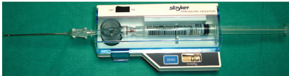
FIGURE 50-4. Intracompartmental pressure monitoring device with digital display.
