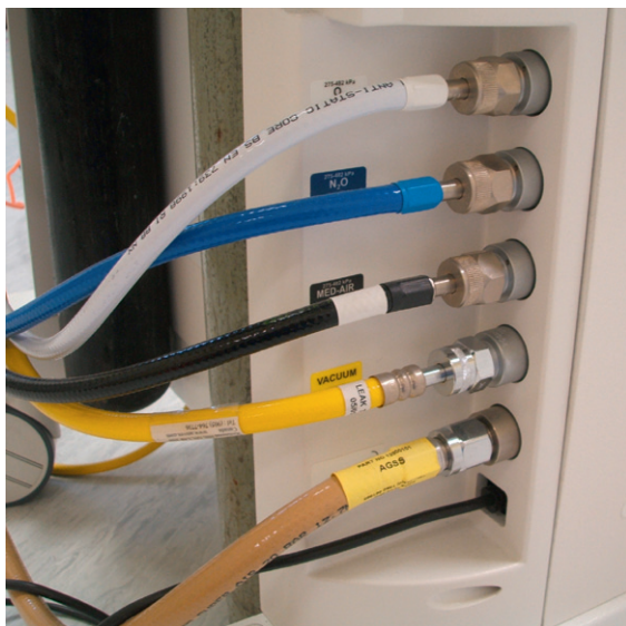
Fig. 1.15 Colour-coded hoses with NIST fittings attached to an anaesthetic machine.
