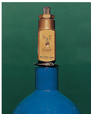
Fig. 1.6 Chemical formula ( N_2O ) engraved on a nitrous oxide cylinder valve.
