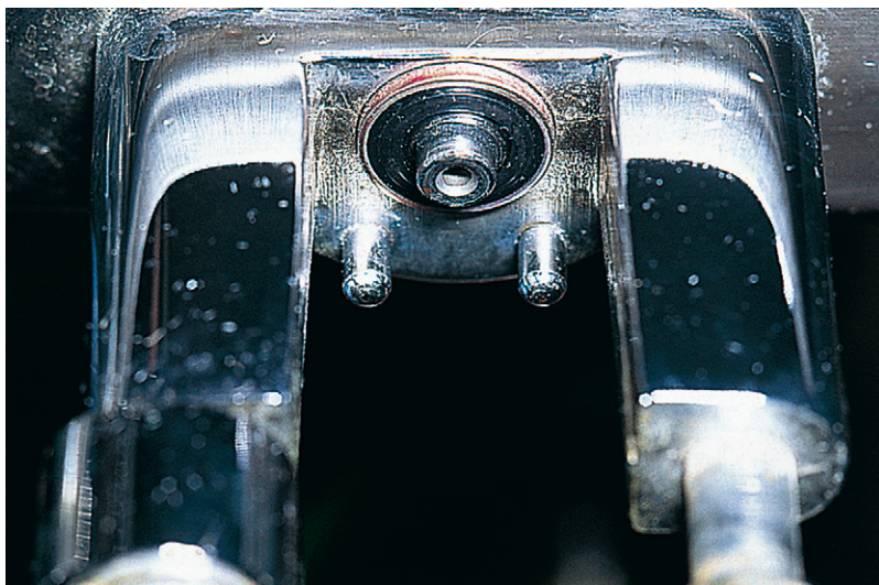
Fig. 1.9 A cylinder yoke and pin-index system. Note that a Bodok seal is in position.
