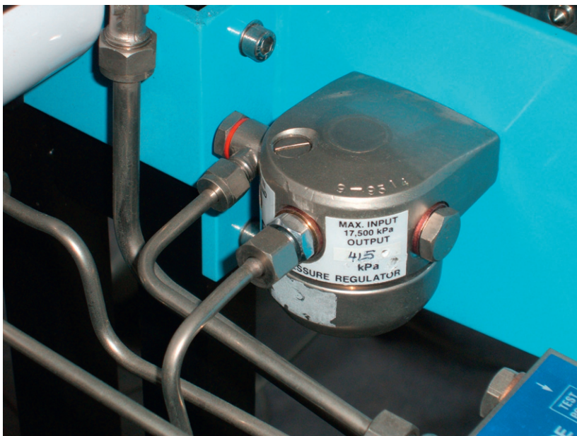
Fig. 2.8 Cylinder pressure regulator (the machine's tray has been removed).
