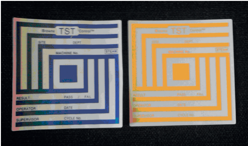
Fig. AppD.3 Bowie Dick test. This is a daily test to ensure that the steam sterilizer is functioning appropriately. Paper patches with heat-sensitive inks are used. The blue patch (left) is a PASS, the yellow patch (right) is FAILED.
