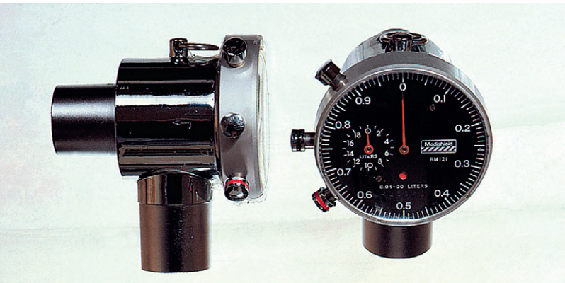
Fig. 10.29 A Wright respirometer. An arrow on the side of the casing indicates the direction of gas flow.
