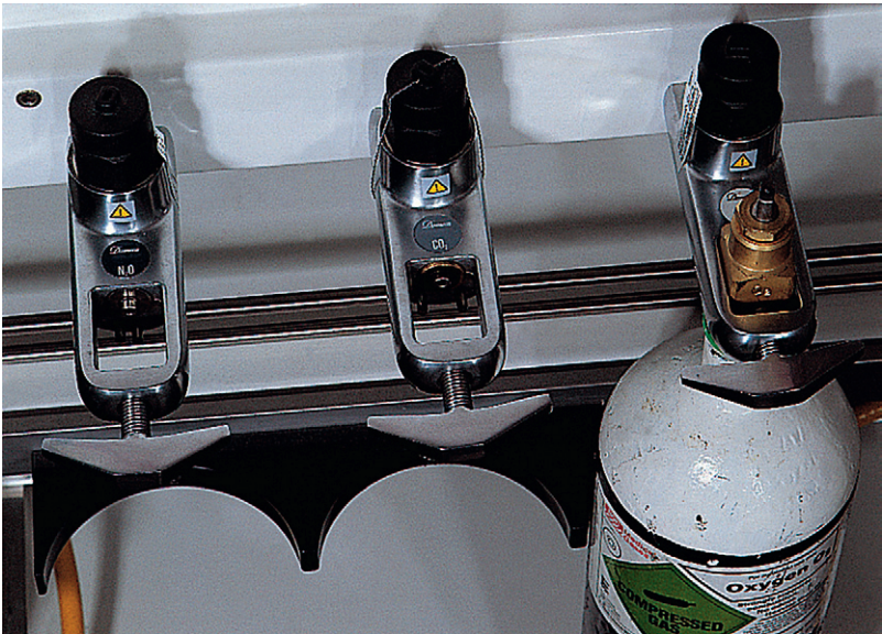
Fig. 1.5 Anaesthetic machine cylinder yokes. For the sake of comparison, the Bodok seal is absent from the nitrous oxide yoke (left).
