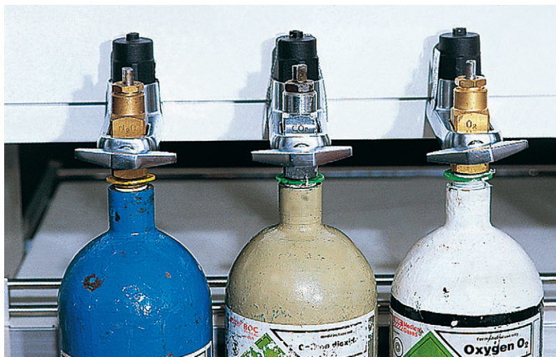
Fig. 2.7 Cylinder pressure regulators (black domes) positioned above the cylinder yokes in the Datex-Ohmeda Flexima anaesthetic machine.
