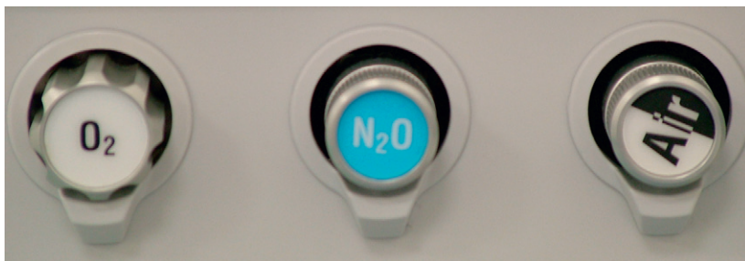
Fig. 2.15 Flow control knobs. Note the colour-coding and the distinctive-shape oxygen control knob.
