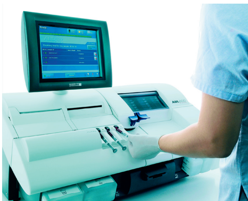
Fig. 13.5 The ABL800FLEX blood gas analyser. (Courtesy of Radiometer Medical ApS.)
