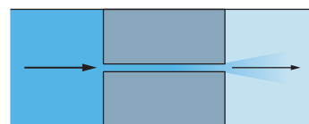
Fig. 2.9 A flow restrictor. The constriction causes a significant pressure drop when there is a high gas flow rate.
