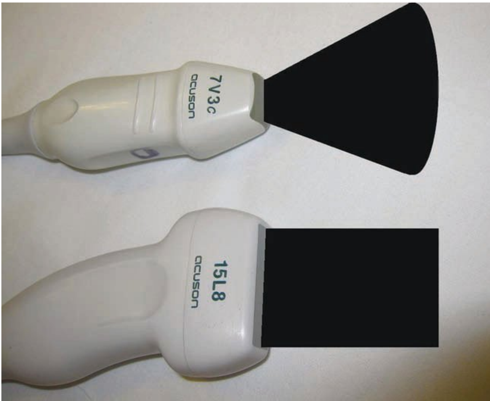
FIGURE 40-22 There are many surface ultrasound probes. For epiaortic ultrasound (EAU) a high frequency is preferable. Shown are a 3- to 7-mHz phased array probe (top) and an 8- to 15-mHz linear array probe (bottom) and the corresponding ultrasound plane shape they can generate. You have to move the actual transducer to scan the area you are interested in, as there are no handle controls, in contrast with the TEE probe.
