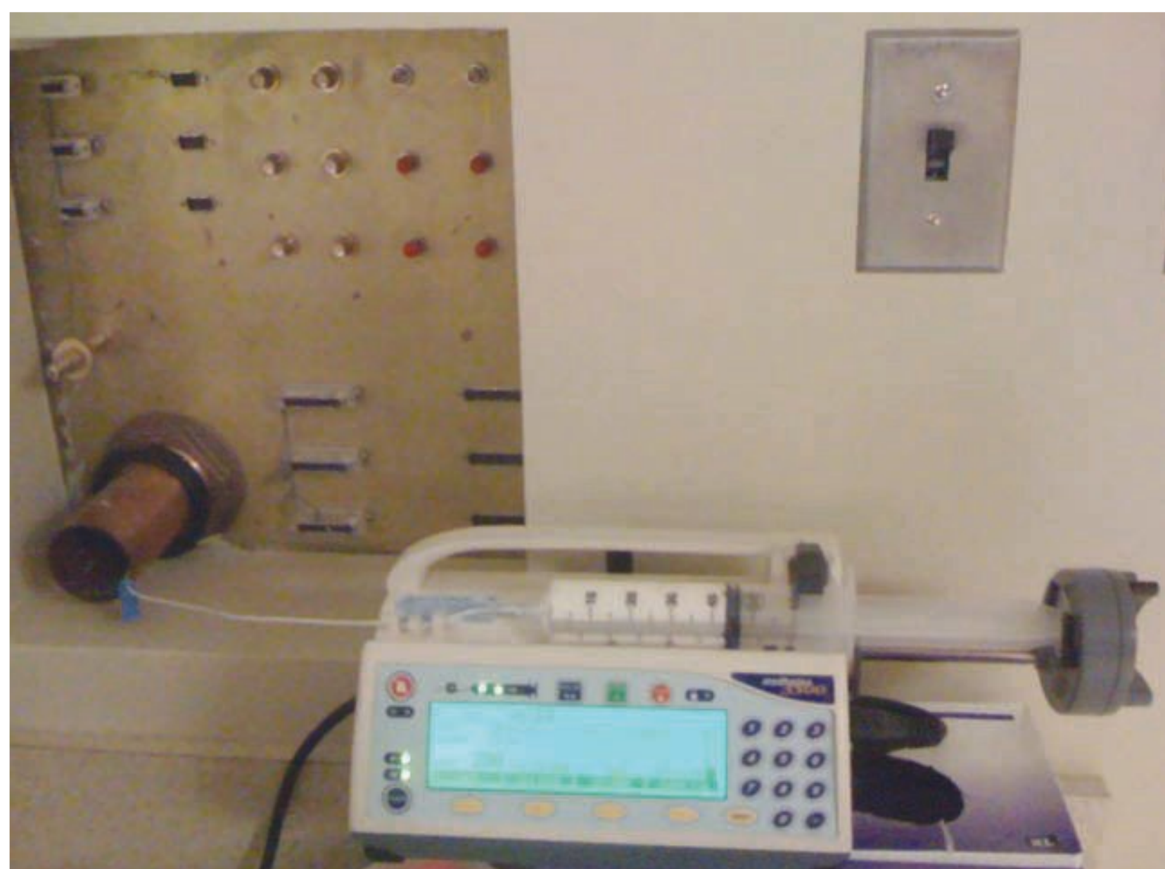
FIGURE 4 6 -5 An infusion pump delivering propofol via extension tubing fed through a copper conduit in the wall to the scanning room.
